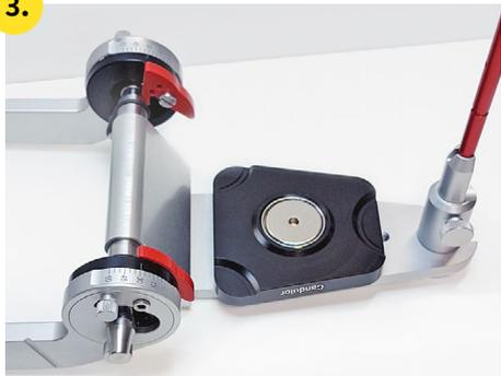
The base plate will be fixed in the upper part of the Candulor plate magnetically, supported by the metal base plate in the articulator and apply metal glue to the center of the plate. Allow the adhesive to cure for at least 90 min. Only then glue the lower plate.
