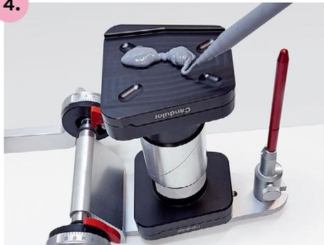
Invert the centring key together with the calibration base plate in the articulator and apply metal glue to the center of the plate.
