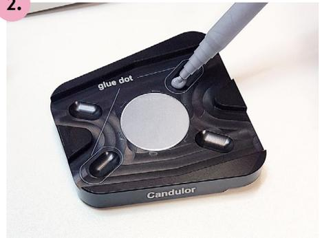
Fill metal glue in the recesses of the base plate marked with "glue dot" and open the articulator, turning it upside-down.
